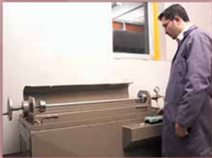
Hidrostatik Test Hydrostatic Test
